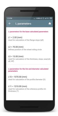
The table displays only those parameters that are necessary for calculating the selected geometric parameters of the wheel (see par. <u>Calculated parameters</u>).
