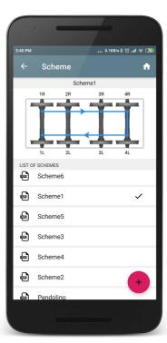
In the figure, the arrows show the direction of measuring the wheelsets, as well as the names assigned to the wheels (1L - first axle, left side; 2L - second axle, left side; 1P - first axle, right side, etc.).
