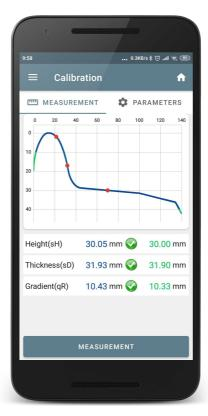
• Tap the **AUTOCALIBRATION** button. The calibration parameters will be automatically calculated and the measured profile will be recalculated.
